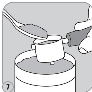
7 Fill the filter with the desired amount of coffee, tamp it lightly, level off and clean the border.
