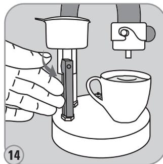
14 Turn the valve slowly to the vertical to flush the residual pressure and stop brewing.
