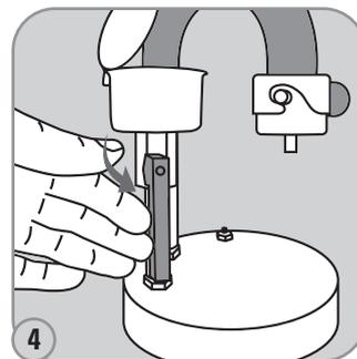
4 Bring the valve to a vertical position to fill the boiler\*.
